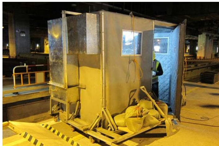
Figure 15: Mobile sound insulation booth
