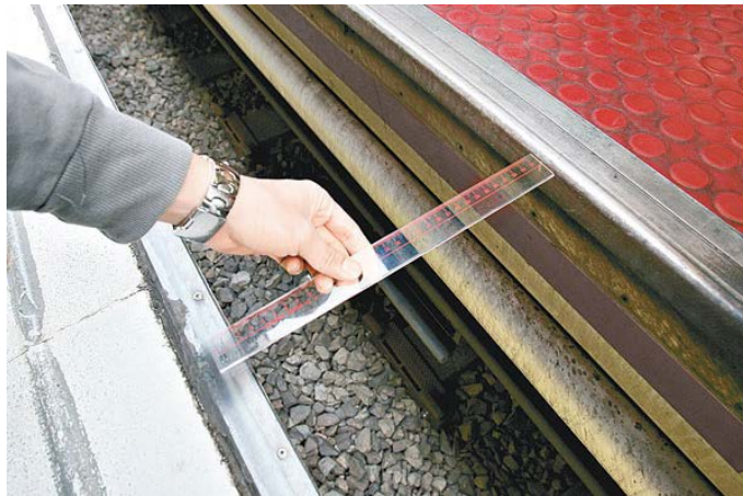
Figure 1: Wide platform gap at an EAL station
